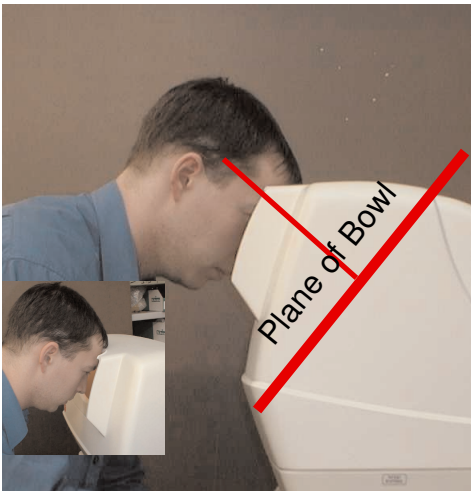
Picture 2 Proper alignment of forehead on brow bar. Inset picture shows alignment for LEFT eye testing.
